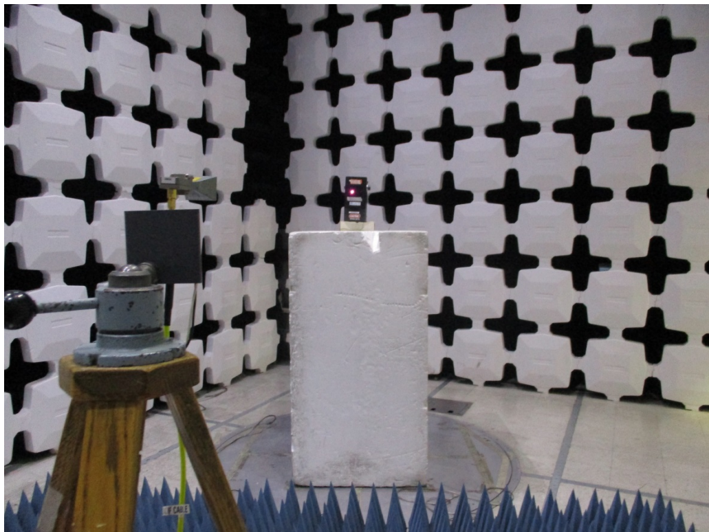
Test Setup for Radiated Emissions, Transmitters– Above 18GHz, Vertical Polarization
