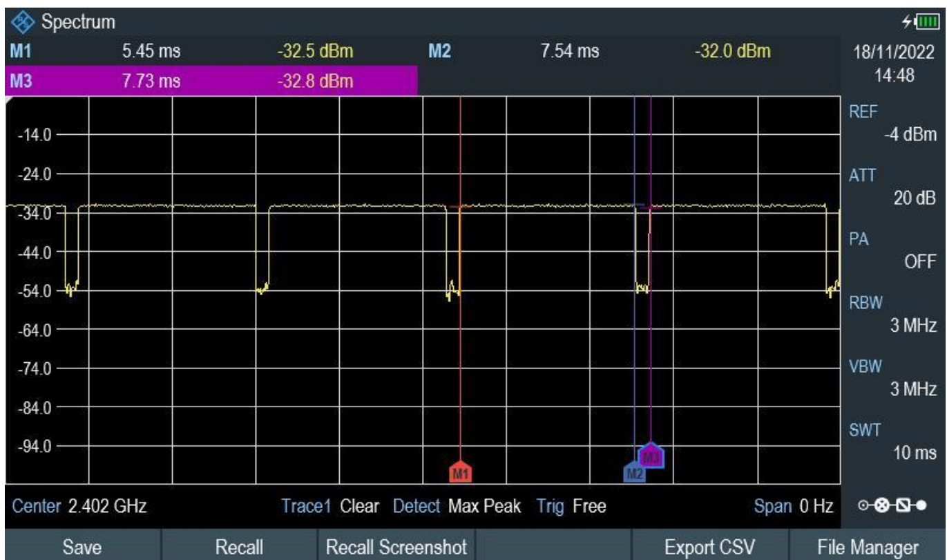
Time-domain plot for Bluetooth transmission signal
