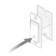
6 Attach the wallplate. Then the wiring is finished.
