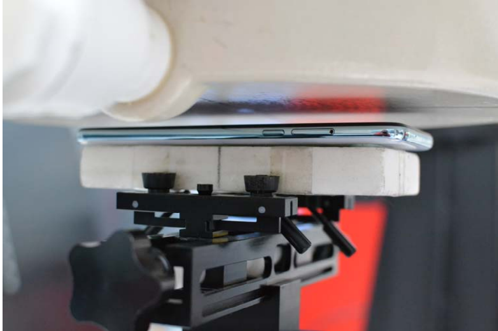
SAR Test Setup Photo 6: Front at 10 mm
