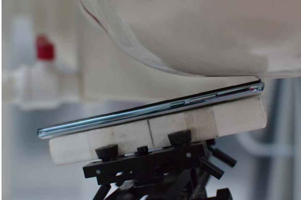
SAR Test Setup Photo 4: Left Tilt
