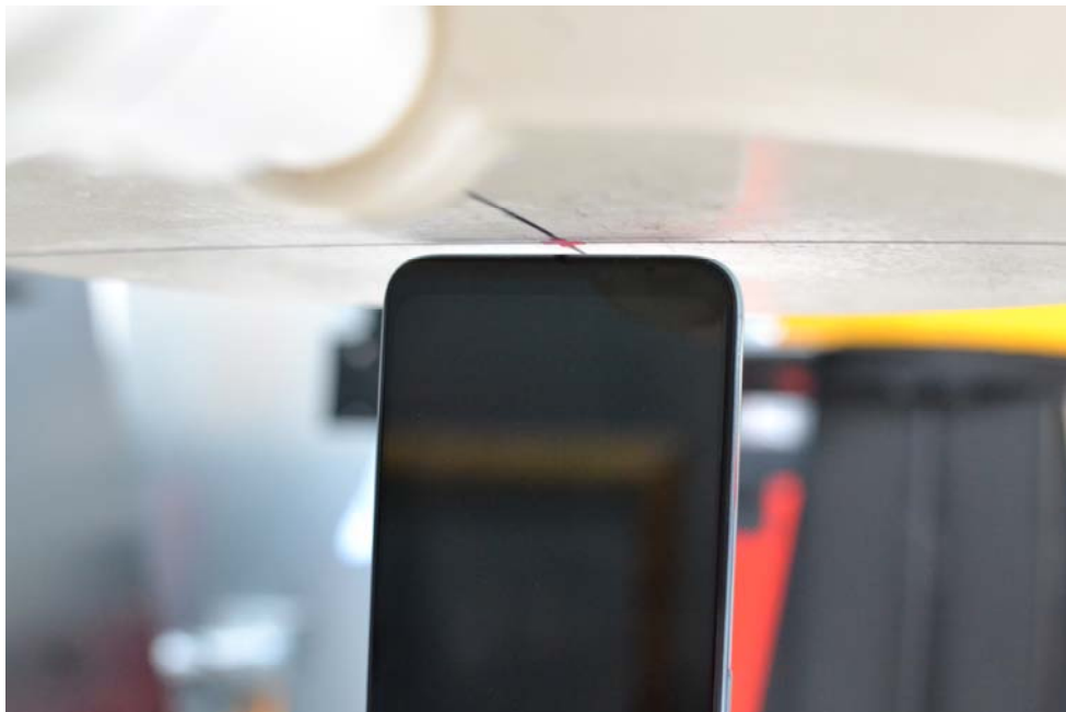
SAR Test Setup Photo 15: Bottom at 3 mm
