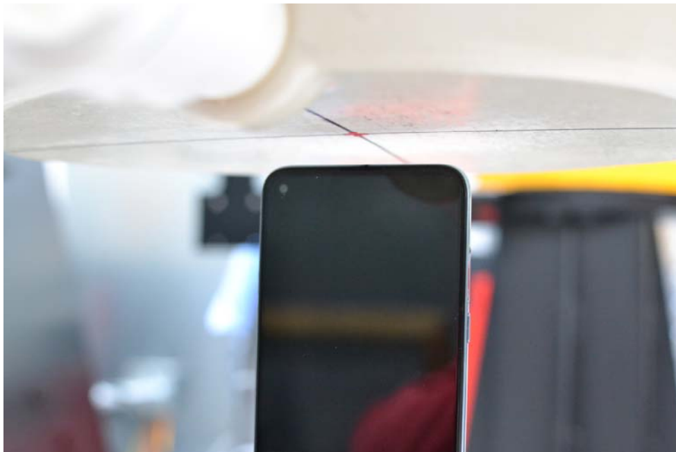
SAR Test Setup Photo 7: Top at 10 mm
