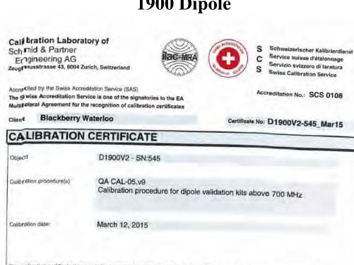
This calibration certificate documents the traceability to national standards, which realize the physical units of measurements (SI) The measurements and the uncertainties with confidence probability are given on the following pages and are part of the certificate.
