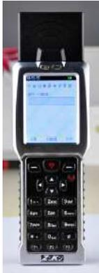
Portable handheld device for user, able to read cards, store data and transmit data through wireless technology to management center.
