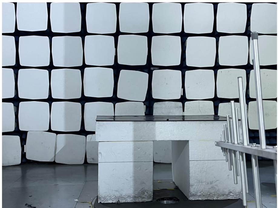
Radiation Emission Test Setup (30MHz to 1GHz)
