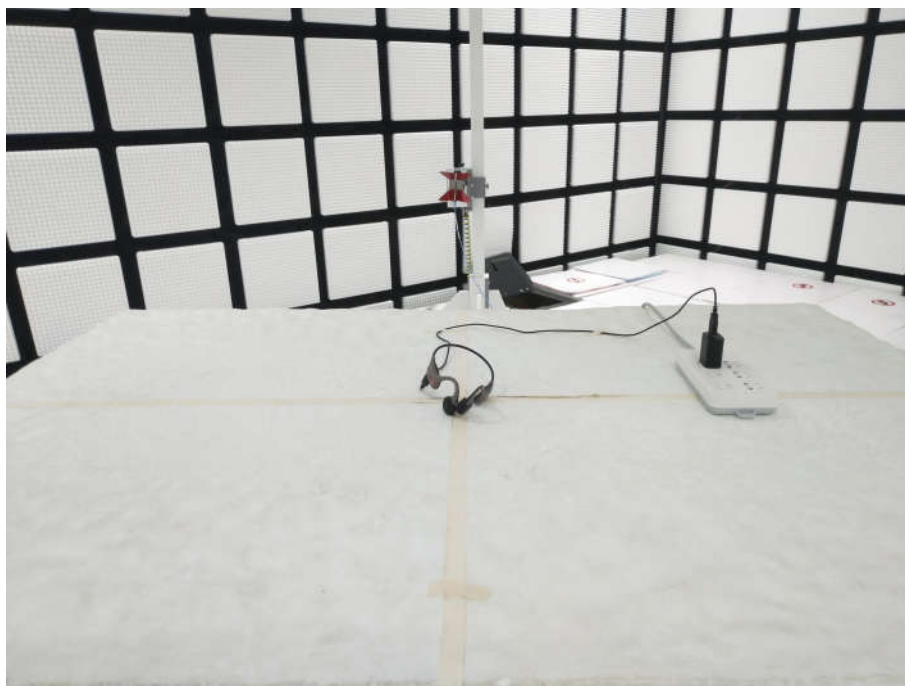
Radiated spurious emission Test Setup-3(Above 1GHz)
