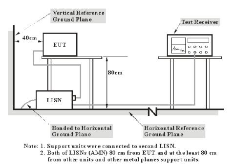
The setup of EUT is according with per ANSI C63.4-2014 measurement procedure. The specification used was with the FCC Part 15 B and Innovation, Science and Economic Development Canada ICES-003 Class B limits..
