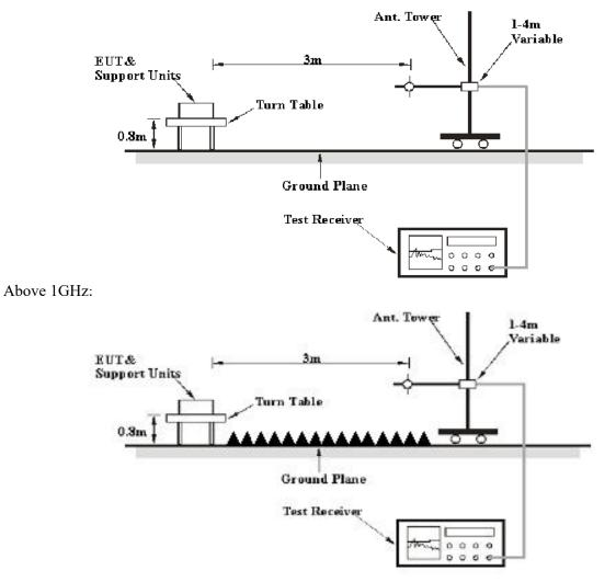
The radiated emission were performed in the 3 meters chamber test site, using the setup accordance with the ANSI C63.4-2014. The specification used was the FCC Part 15.109 and ICES-003 Class B limits.
