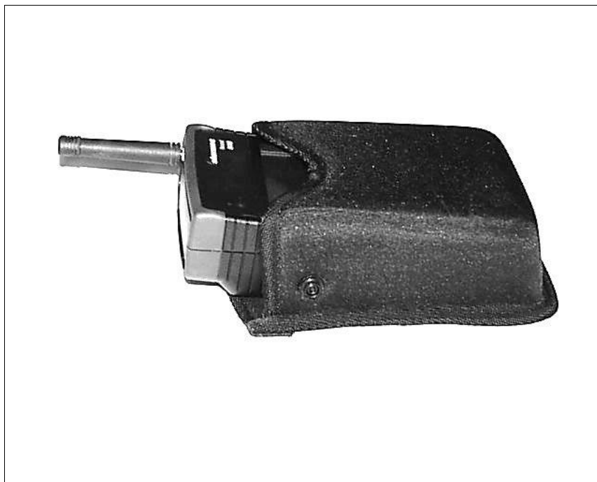
Photo 6: Shows close-up of 6100 forward within the pouch with antenna away from the operator.
