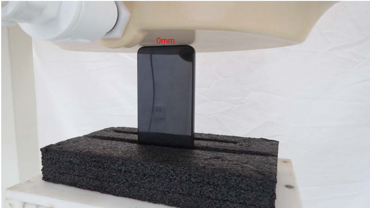
Picture 13: Bottom Edge, the distance from handset to the bottom of the Phantom is 0mm
