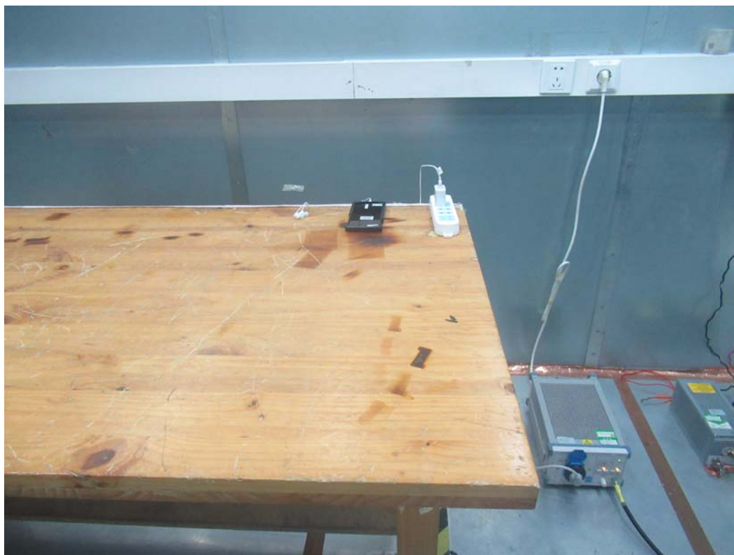
Picture 2 Conducted Emission Test Setup
