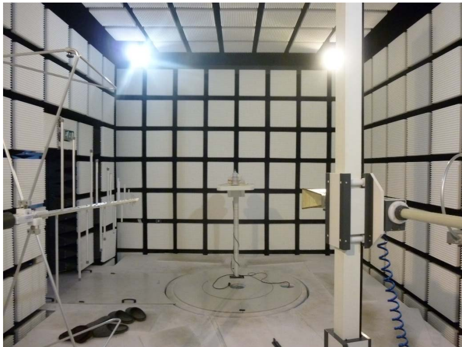
Photo 6: EUT at the anechoic chamber
