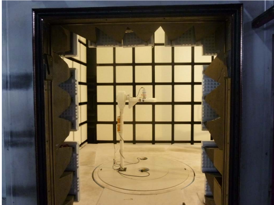
Photo 1: EUT at the anechoic chamber
