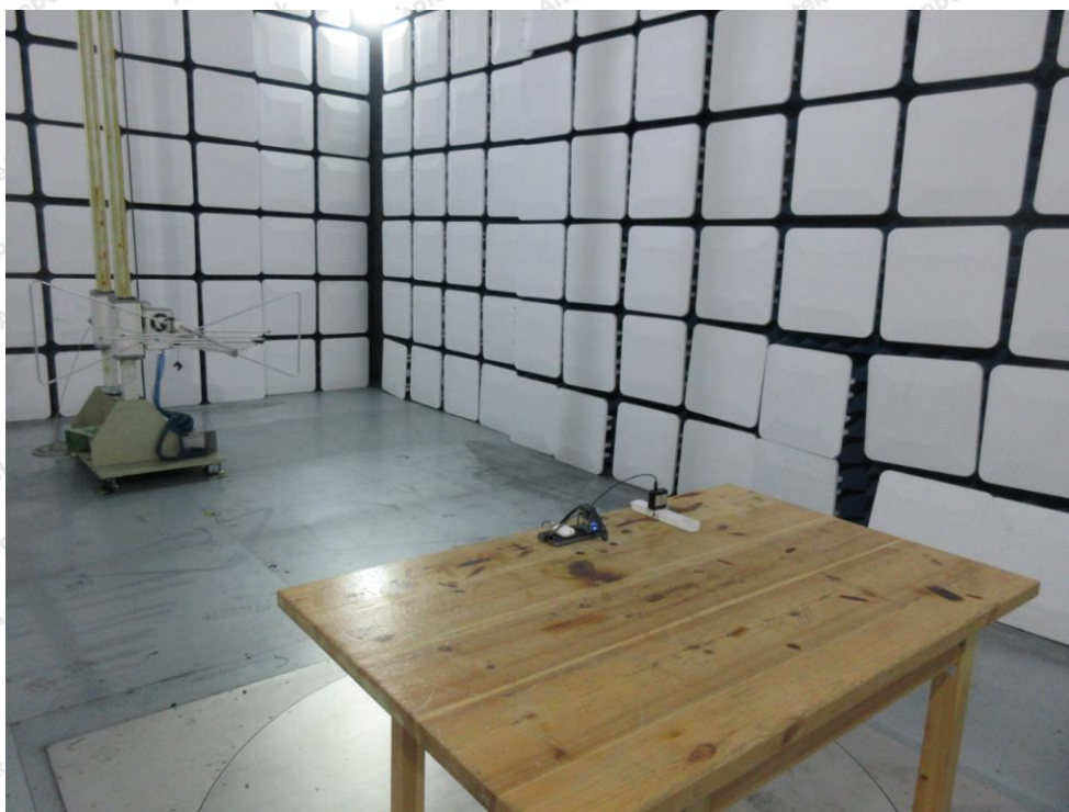
Photo of Radiation Emission Test
