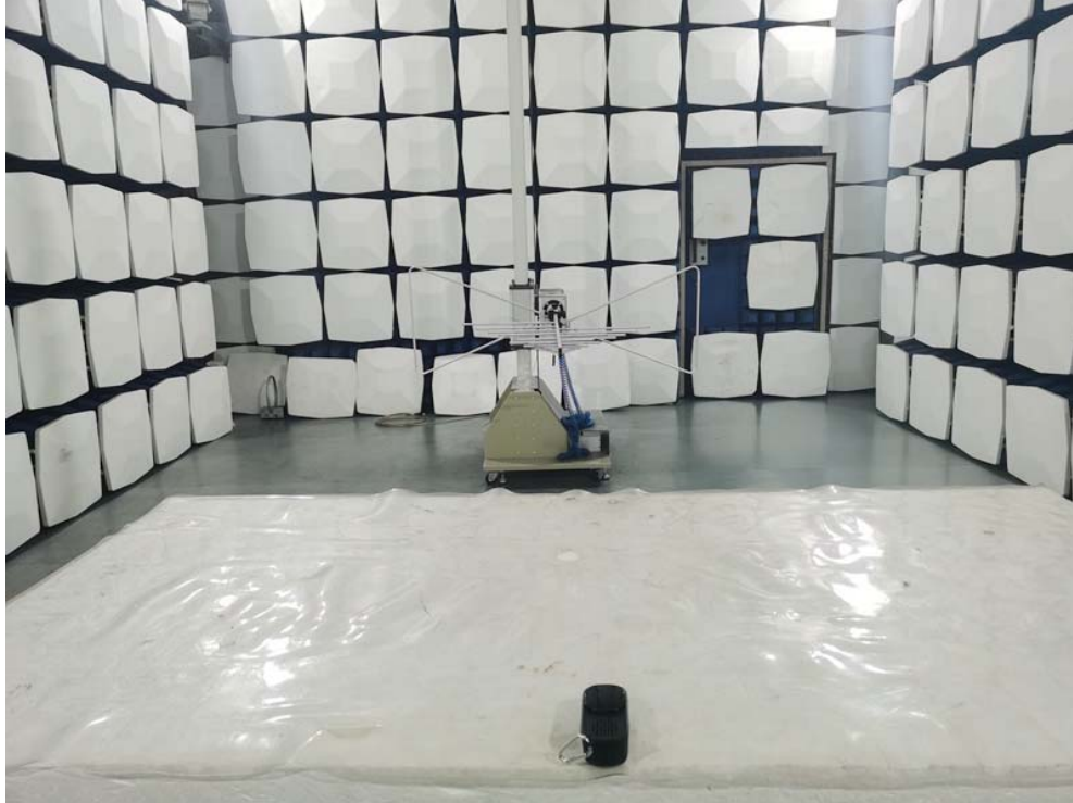
Radiated Emission Test Setup:
