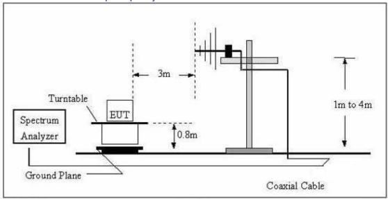
(C) Radiated Emission Test-Up Frequency Above 1GHz
