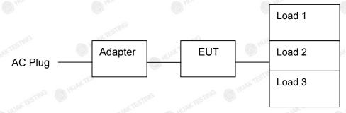
Operation of EUT during radiation above 1GHz testing:
