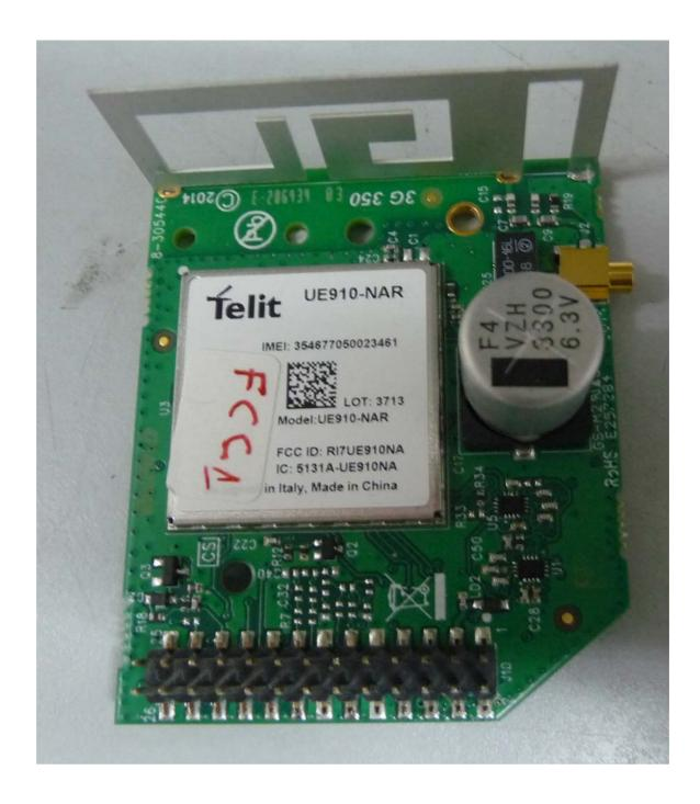
Photograph No.17 Control panel 2G/3G module second side view
