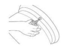
Break the bead of the tire ensuring the valve is located on Place the valve through the valve hole, ensuring the rubber the opposite side of the rim from the bead breaker blade, grommet makes good contact with the valve hole all around. When the tire is dismounted the valve must be located at 1 o'clock to the tire fitting head.
