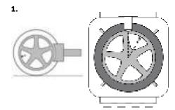
Break the bead of the tire ensuring the valve is located on the opposite side of the rim from the bead breaker blade. When the tire is dismounted the valve must be located at 1 o'clock to the tire fitting head.
