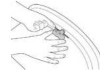
Place the anti-rotation pin into the valve hole to prevent movement of the sensor during tightening.
