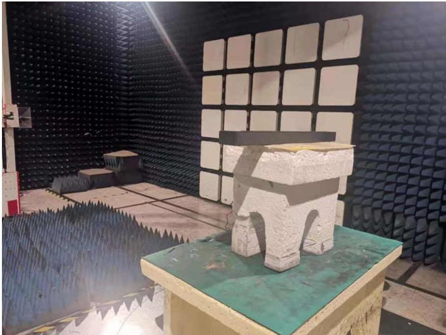
Spurious Emission Test Setup (Above 1GHz)
