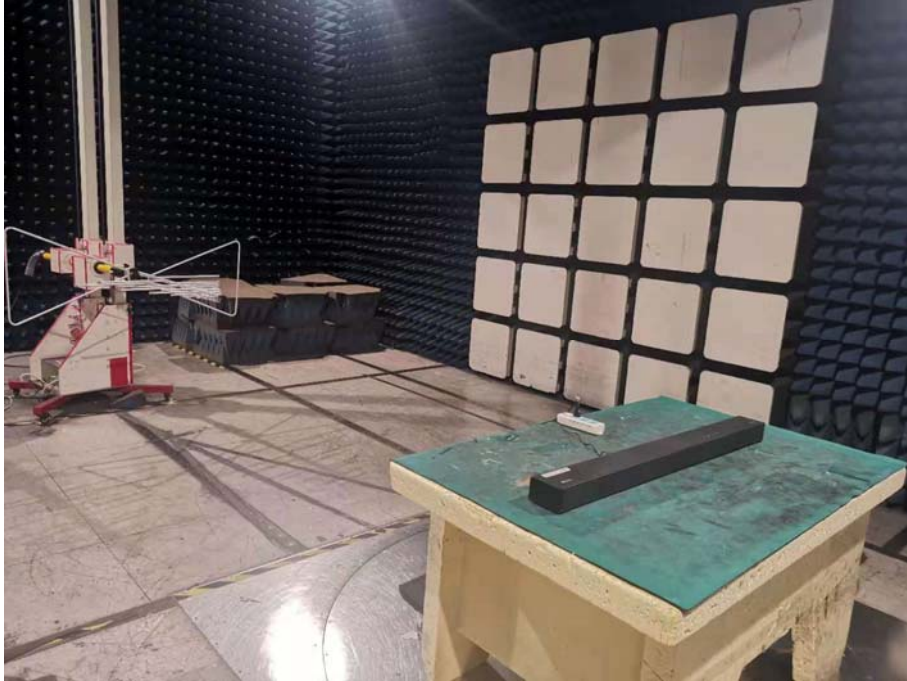
Spurious Emission Test Setup (Above 1GHz)
