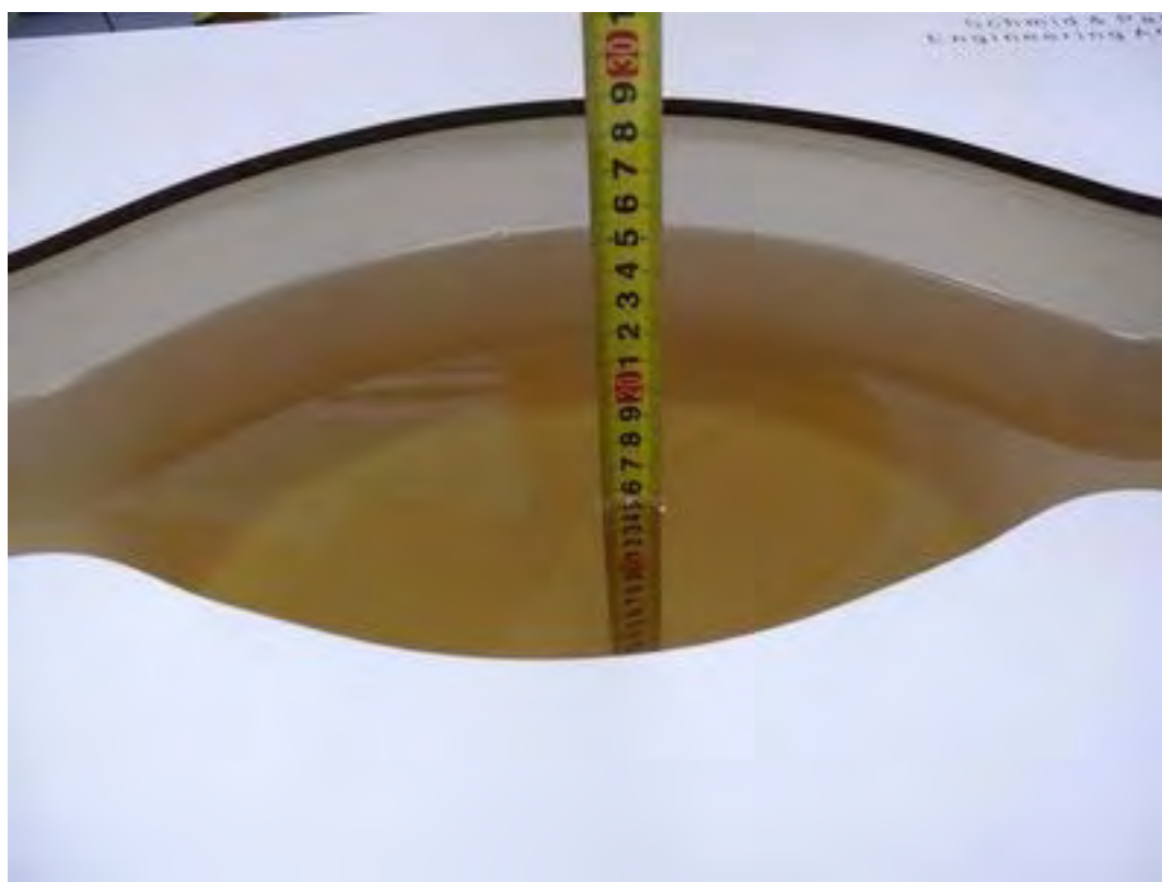
Picture 4: Liquid depth in the flat Phantom (750MHz, 15.4cm depth)
