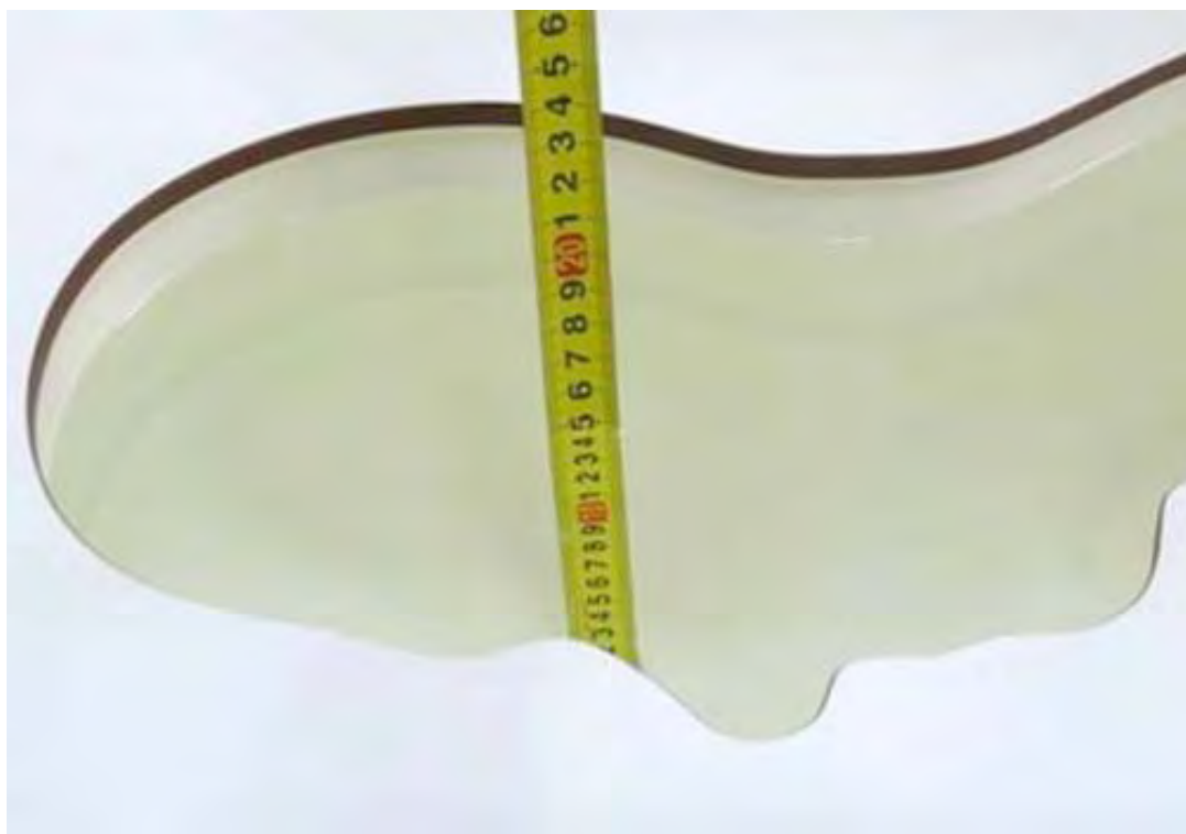
Picture 15: Liquid depth in the head Phantom (5250 MHz, 15.4cm depth)
