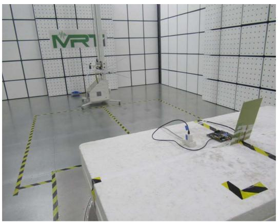
Description: Transmitter Spurious Emissions Test Setup for 1GHz ~ 18GHz
