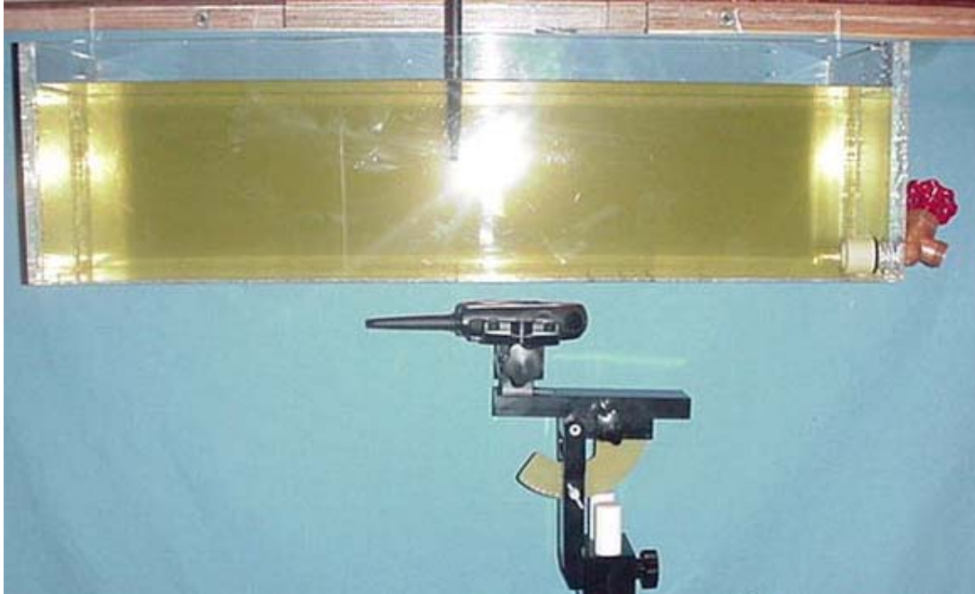
Face-Held SAR Test Setup Configuration
