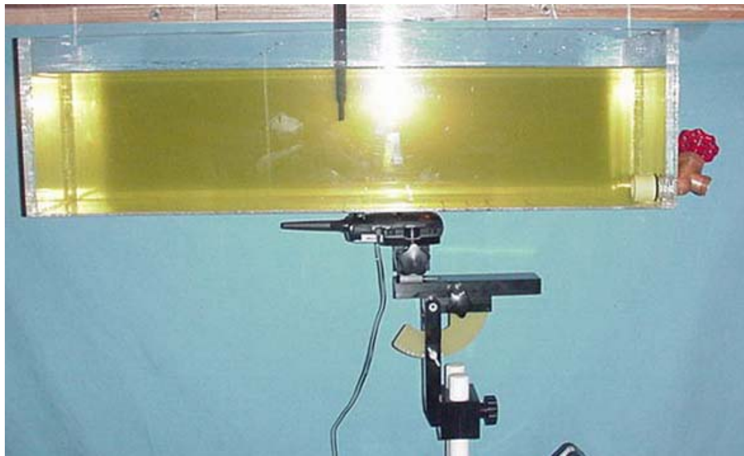
Body-Worn SAR Test Setup Configuration
