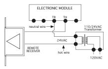
Connect the neutral wire from the 24VAC transformer to the TR (transformer) terminal on the ELECTRONIC MODULE. Connect the hot wire from the 24VAC transformer to either of the wire terminals on the remote receiver. Connect another wire (included) between the other receiver wire terminal and the TH (thermostat) terminal on the ELECTRONIC MODULE.
