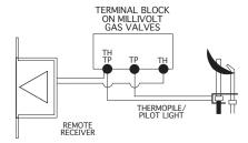
Installer must connect two 18 gauge wires from the remote receiver to the TH and TH/TP terminals on the millivolt gas valve. (It does not matter which receiver wires are connected to the designated terminals listed above.)
