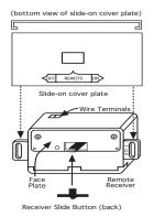
The remote receiver can be placed on the fireplace hearth or under the fireplace, behind the control access panel, or on any space heating appliance.
