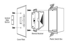
Install four 1.5V AA-size ALKALINE batteries (Included) in the remote receiver. For best performance, remote receiver batteries should be factory fresh when installed. Very little battery power is required to operate the remote receiver, but the electronics are tuned to operate best when battery output is greater than 5.3 volts. For new AA batteries should provide an output voltage of 6.0 to 6.2 volts.
