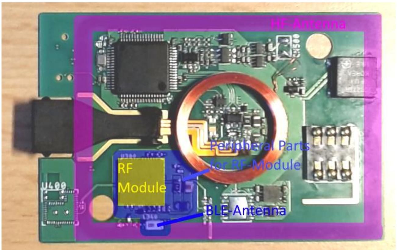
Picture 1: Description of BLE module and evaluation board
