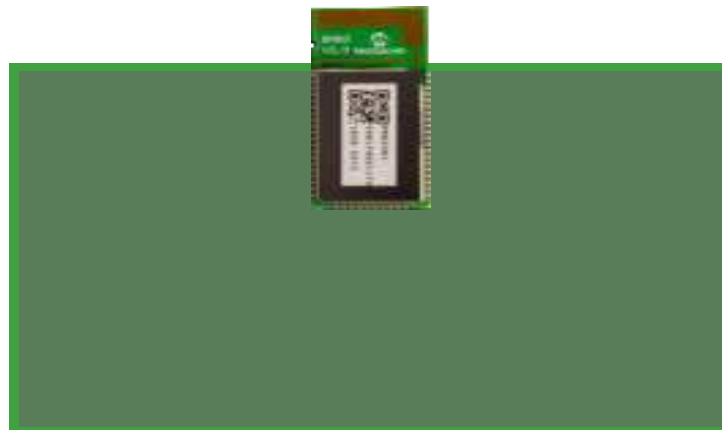
Figure 7-5. Recommended Module Placement
