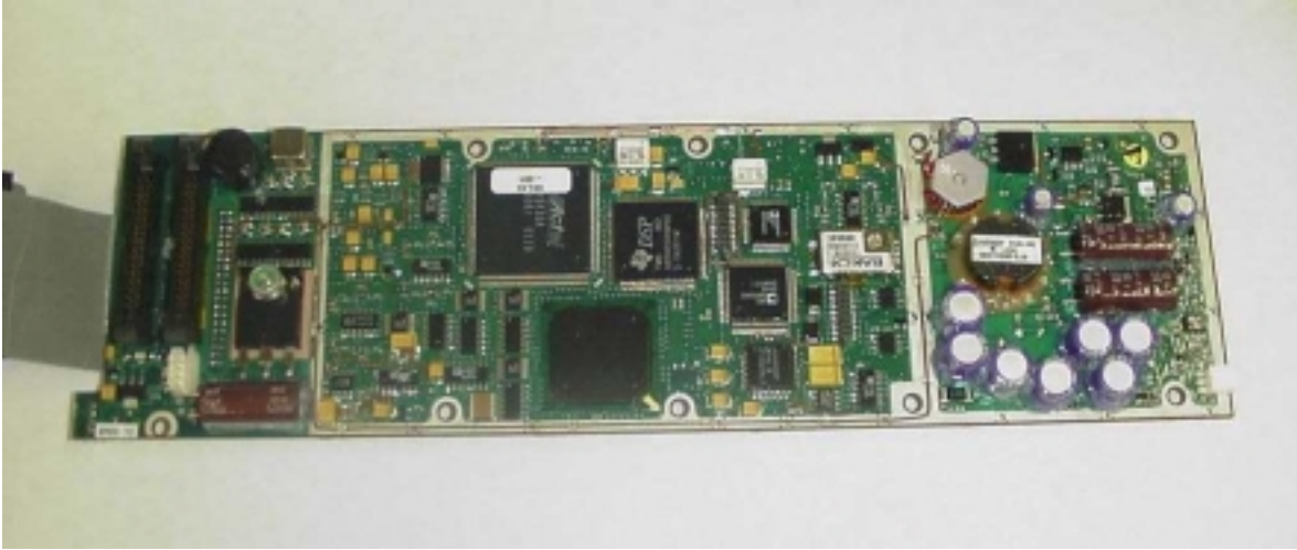
Photo 1: DSP/Power Supply Circuit Card, Top View
