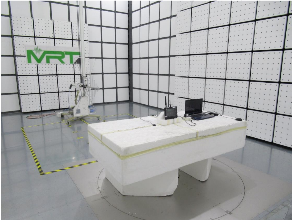
Description: Radiated Emission Test Setup for 1GHz~18GHz
