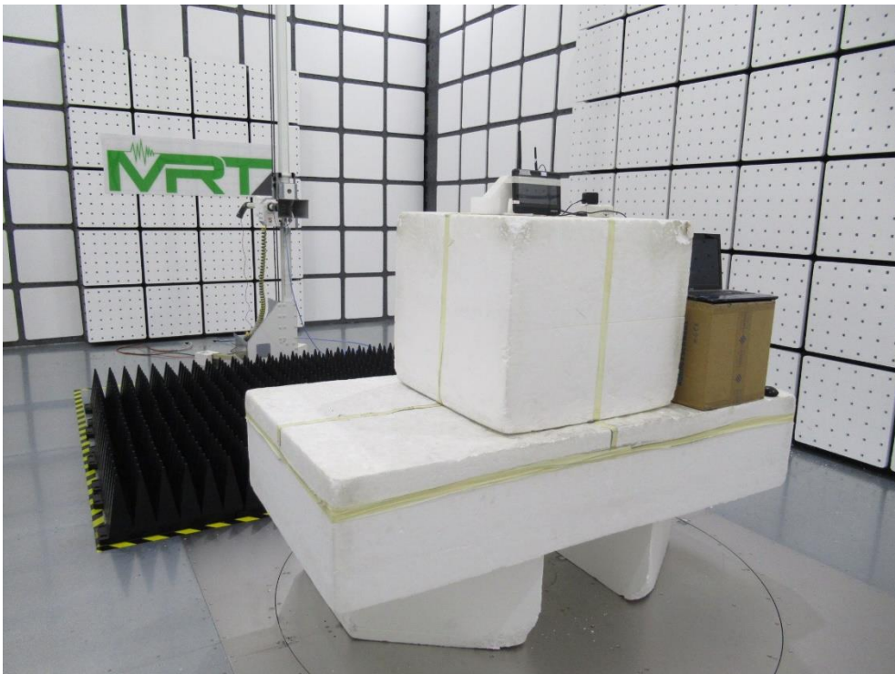
Description: Radiated Emission Test Setup for 1GHz~18GHz
