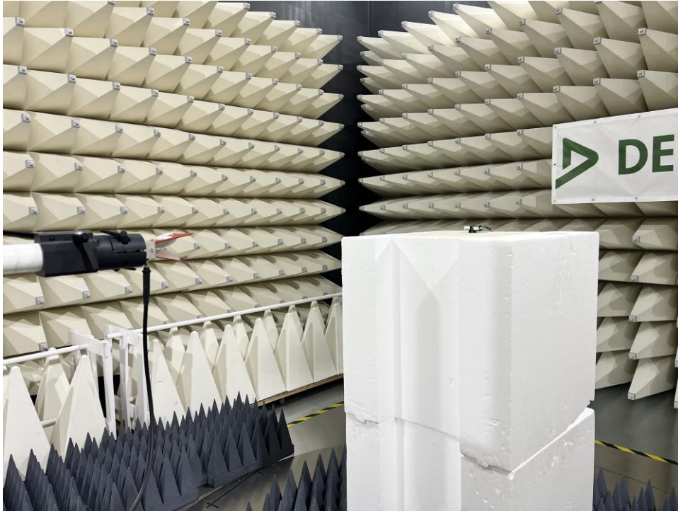
Figure B7. High Range Radiated Emission test setup 2
