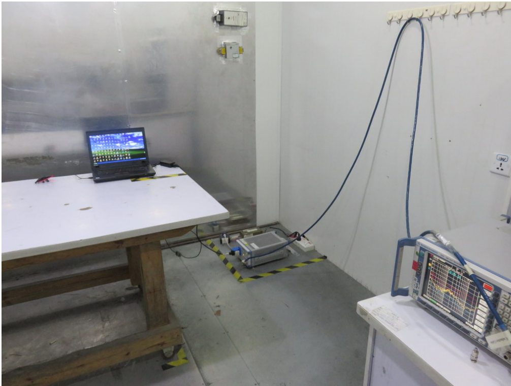
FCC RADIATED EMISSION TEST SETUP
