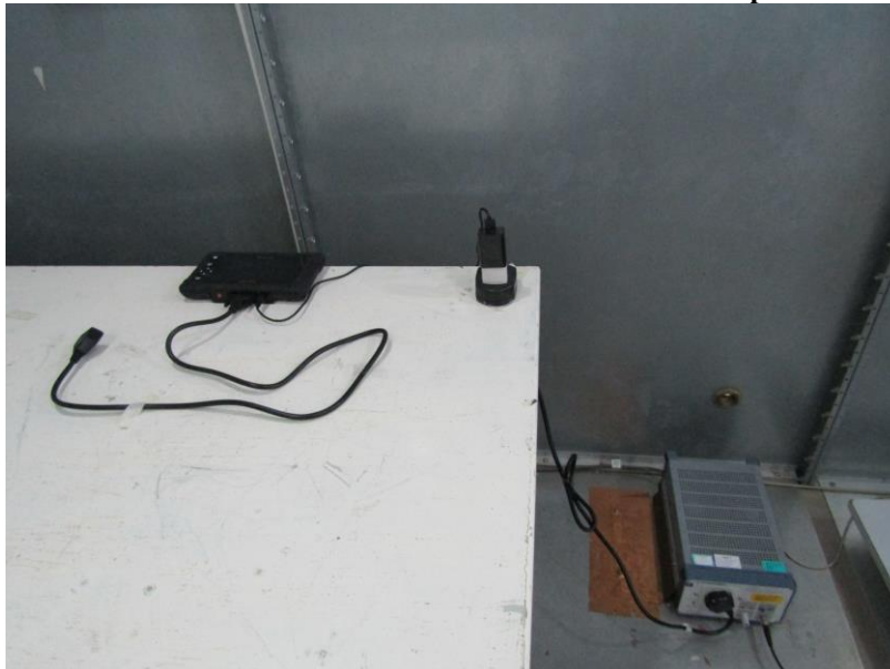
Measurement of Conducted Emission Test Set Up
