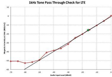
This model was verified to be within the linear region for ABM1 measurements at -16 dBm<sub>0</sub> for GSM, UMTS, and VoLTE over IMS. This measurement was taken in the axial configuration above the maximum location.
