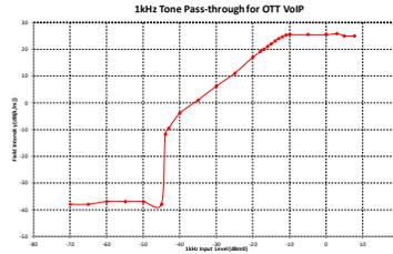
This model was verified to be within the linear region for ABM1 measurements at -20 dBm<sub>0</sub> for VoWiFi over IMS and OTT VoIP. This measurement was taken in the axial configuration above the maximum location.
