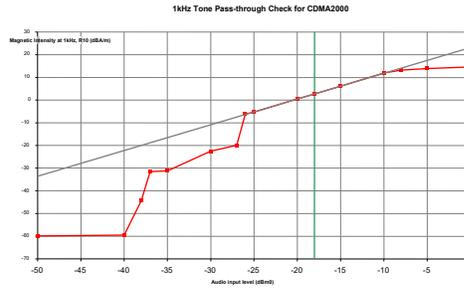
This model was verified to be within the linear region for ABM1 measurements at -18 dBm<sub>0</sub> for CDMA. This measurement was taken in the axial configuration above the maximum location.
