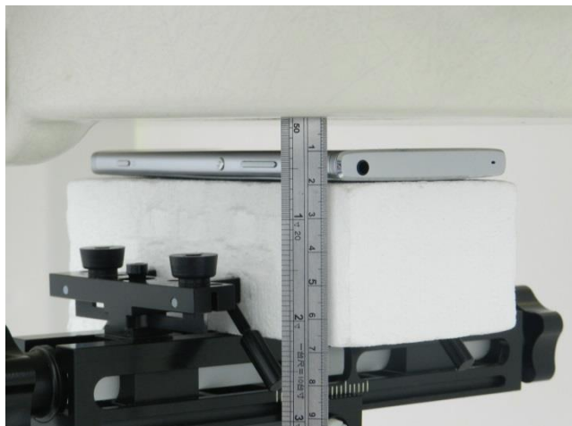
Front, Test Separation 10 mm
