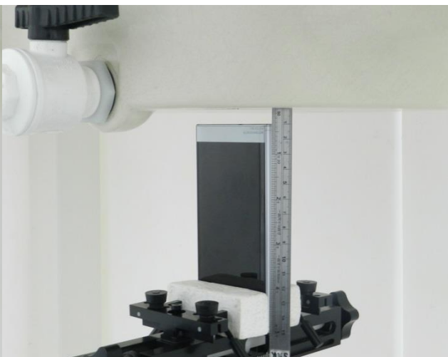
Bottom Side, Test Separation 10 mm
