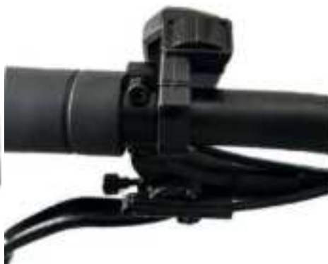
4. Check whether the brake handle, headlight switch, dual drive switch, and instrument are fixed
