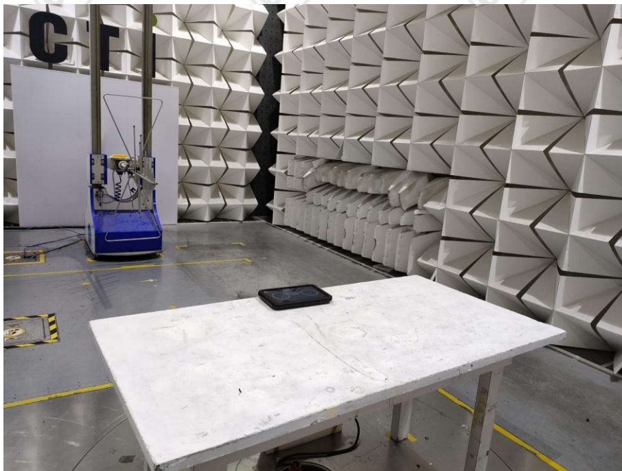
Radiated spurious emission Test Setup-1(Below 1GHz)
