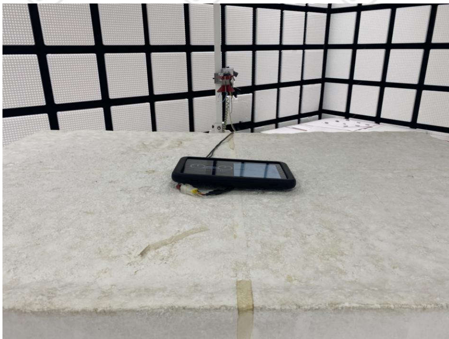
Radiated spurious emission Test Setup-2(Above 1GHz)
