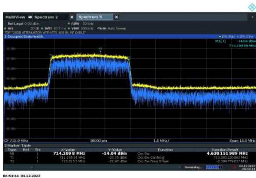
LTE B12 Uplink High Channel OBW @ 20°C Nominal Voltage
