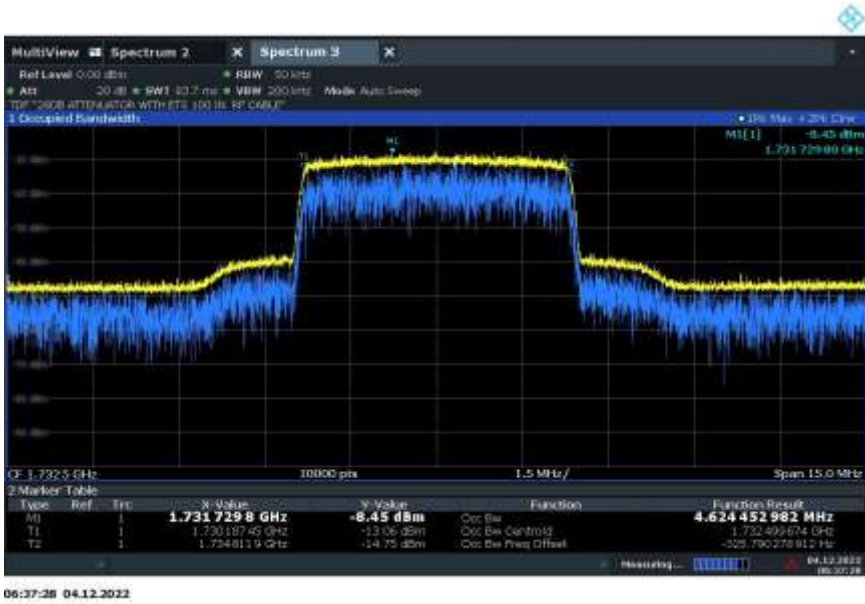
LTE Band 4 Uplink Middle Channel OBW 120VAC @ 20°C
