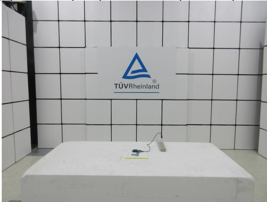
Photograph 2: Test Setup for Spurious Emissions (Front View 2)
