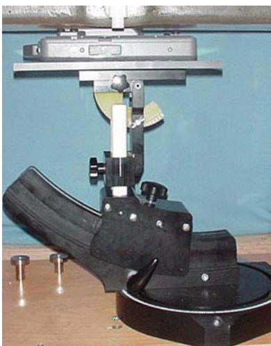
DUT Test Setup with External 2 nd Battery
