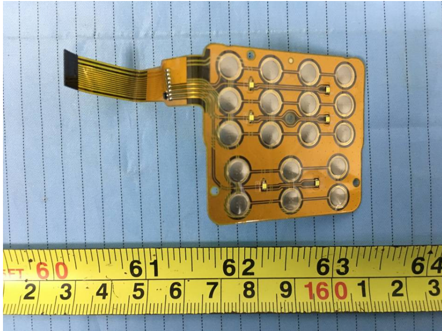
EUT –FPC keyboard Top View
