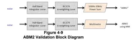
The power summed output results for a known input were compared to the multi-meter results to verify any deviation in the post-processing implemented with the power-sum.
