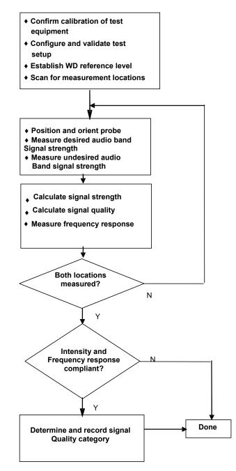
Figure 4-15 C63.19 T-Coil Signal Test Process
