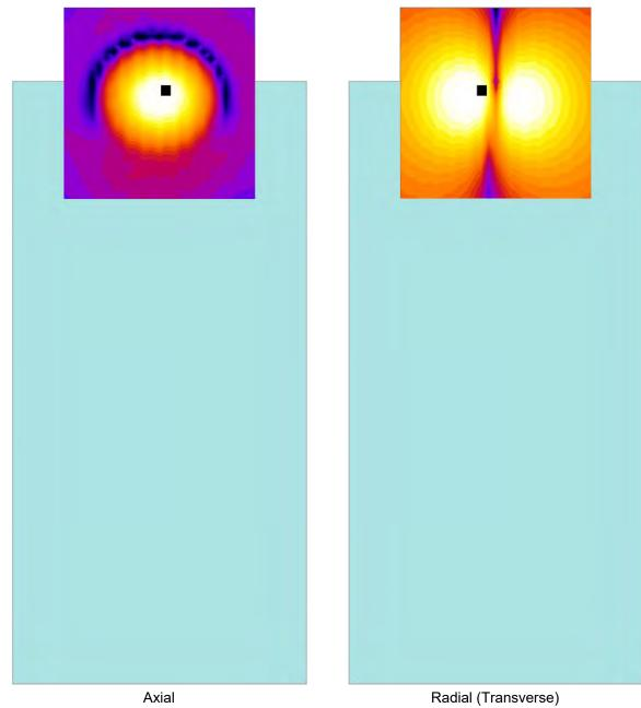
Figure 9-1 T-Coil Scan Overlay Magnetic Field Distributions
