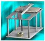
**Figure 4-3** RF Near-Field Scanner
