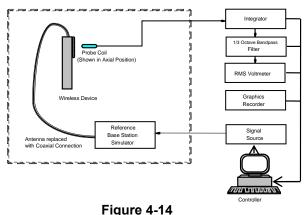
Audio Magnetic Field Test Setup
