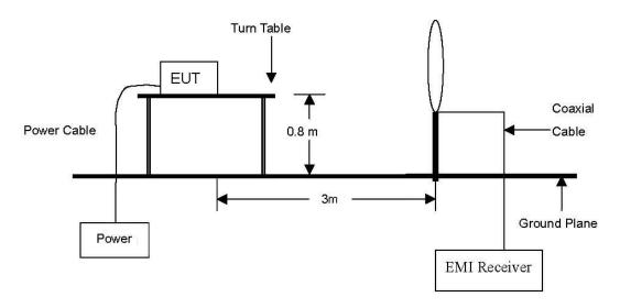
The diagram below shows the test setup that is utilized to make the measurements for emission from 30  $\,\mathrm{Mz}$  to 1  $\,\mathrm{GHz}$  emissions.
