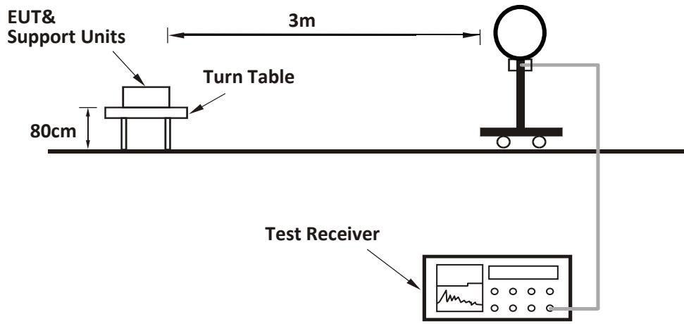
For Radiated emission 30MHz to 1GHz:
