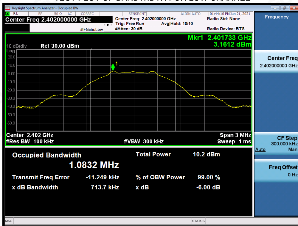
TEST PLOT OF BANDWIDTH FOR LOW CHANNEL
