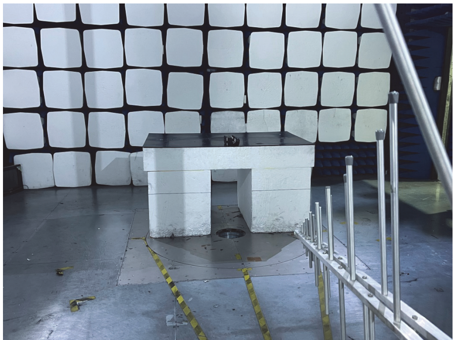
Radiation Emission Test Setup (30MHz to 1GHz)
