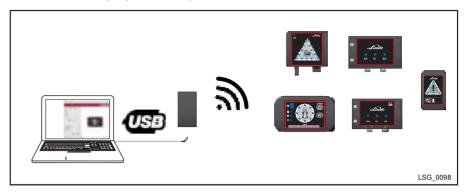
Use the additional USB-Cable to connect the programmer to your computer. With the software tool "Wireless Flasher", the programmer enables you to send new firmware to the devices. Furthermore, the provided configuration tool enables the service technician to configure the signaling zones.
