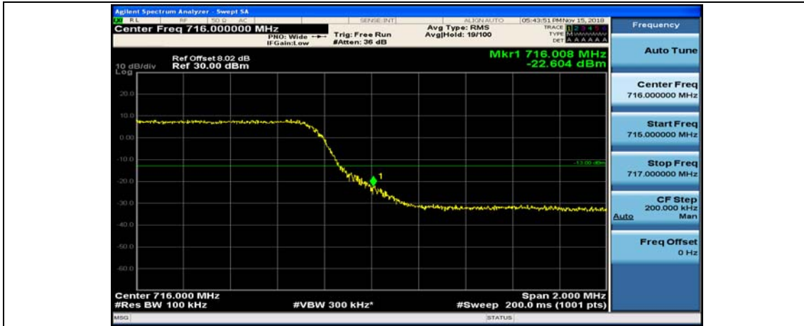
(Channel Bandwidth: 5 MHz)_LCH_16QAM_1RB#0
