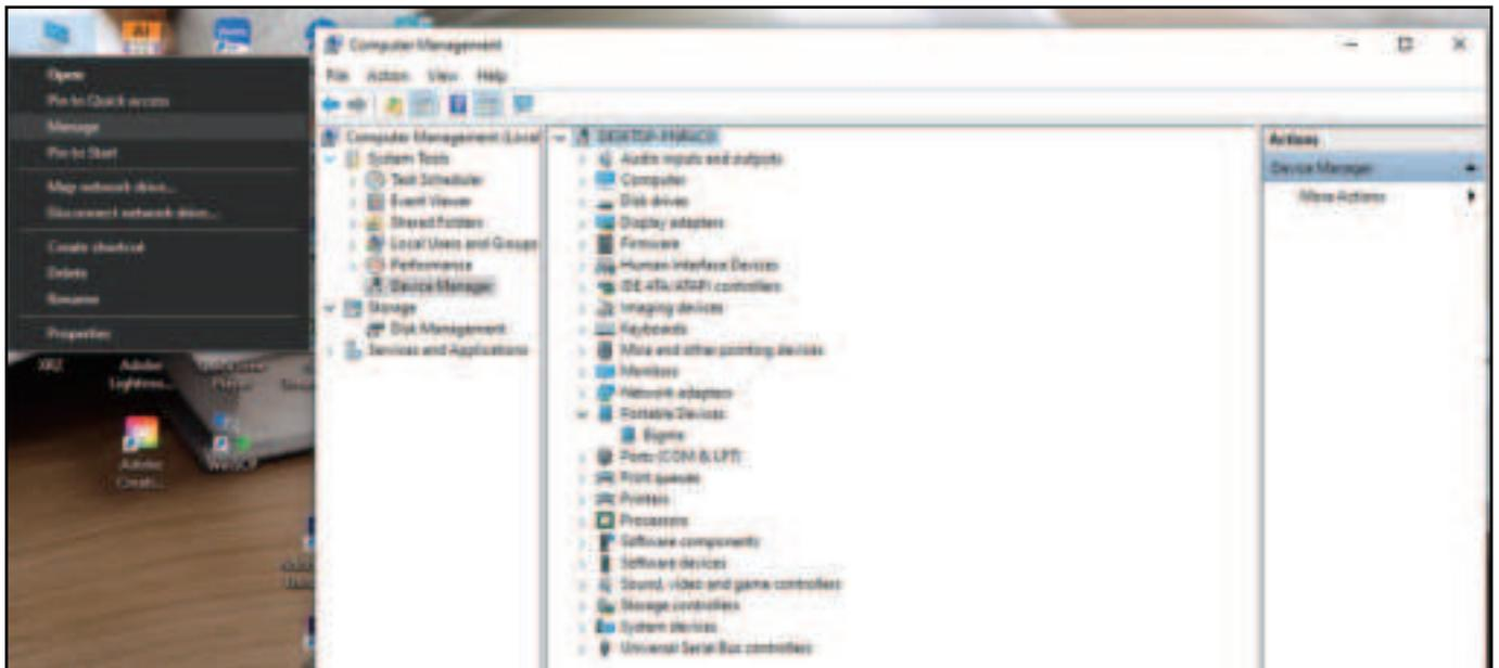
1. After the device is connected to the computer, right-click on the computer desktop [This PC], select [Manage] > [Device Manager] > [Portable Device-Bigme]
