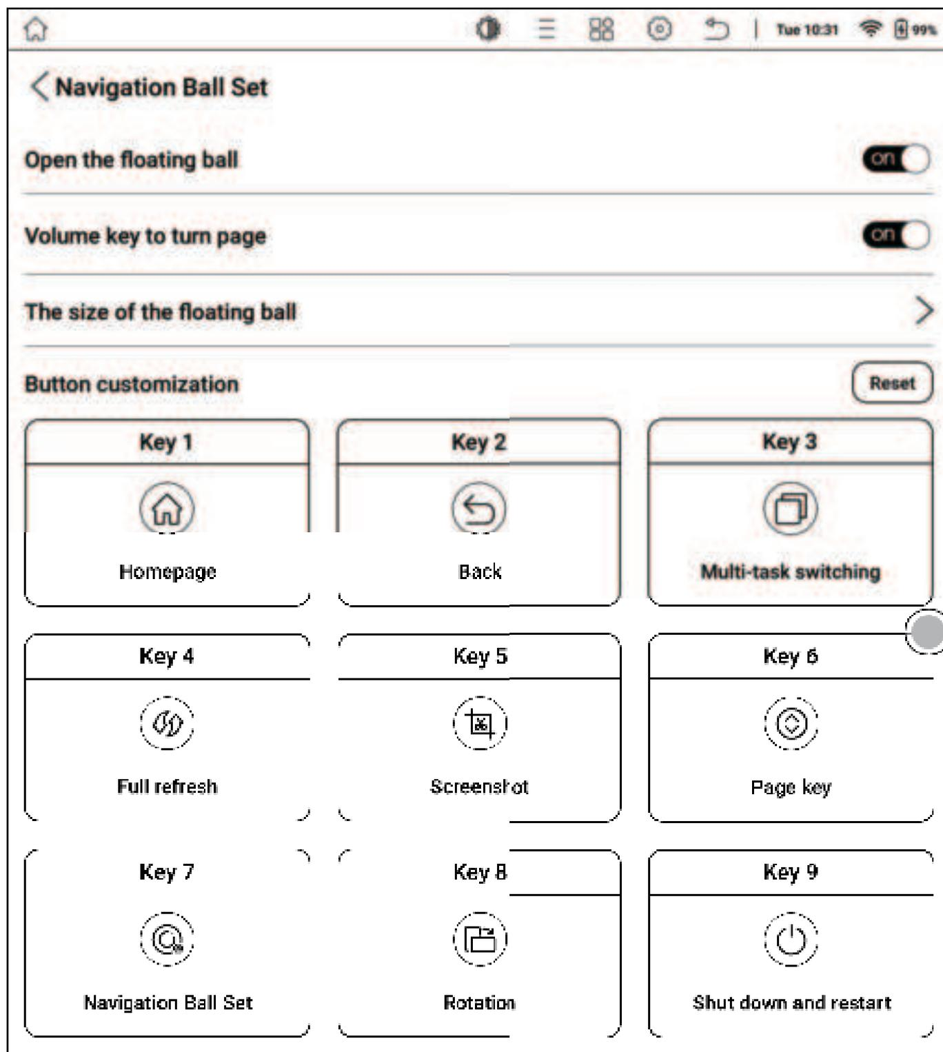
1. A control menu that floats on the top layer of the interface, you can customize the settings for 9 button functions
