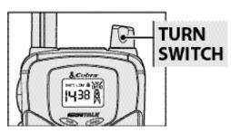
**1** Turn the On/Off/Volume switch. An audible "tone" will indicate the unit is on.
