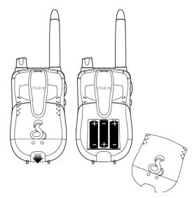
• Pull lock tab down to remove battery cover.
