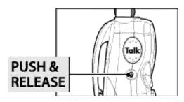
Push and release LIGHT/MAX RANGE button to illuminate display for ten seconds.
