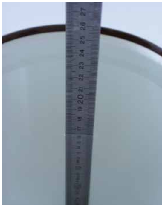
Fig. 18: Liquid depth for 2450 MHz Head measurements.
