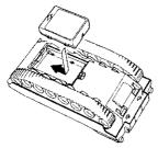
③ Install the Ni-Cd cassette pack in the battery compartment as shown in the diagram. The Ni-Cd cassette pack is designed so that the + and - poles must be positioned properly or else the pack cannot be installed.
