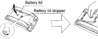
① Turn the battery lid stopper with a coin, as ② Pull up the battery lid to open. shown in the diagram.
